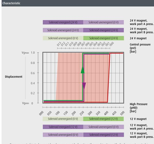
Pressure control is to be considered as an override function. If a combination with displacement control is applied, this function, also known as the basic control function, is overridden by pressure control within the corresponding control range.
