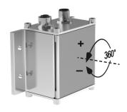
The definition of the measurement axis is indicated on the device. For the standard installation position, TOP4@x-axis, and signal path CCW this is depicted below. The position signal is zero (360°  $\rightarrow$  0°) in this configuration when the connectors point upwards. Due to the preset function other zero positions are adjustable by the customer.
