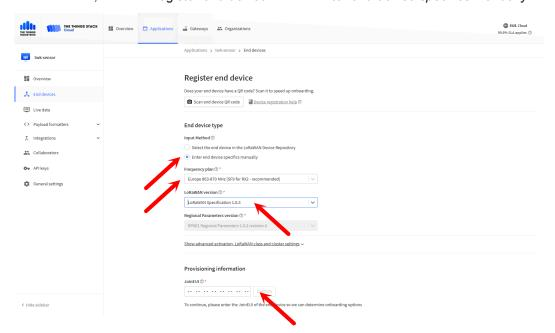
Under Frequency plan select Europe 863-870 MHz (SF9 for RX2 - recommended). Under LoRaWAN version, select LoRaWAN Specification 1.0.3. Enter the JoinEUI, which can be found on the device. Click confirm.
