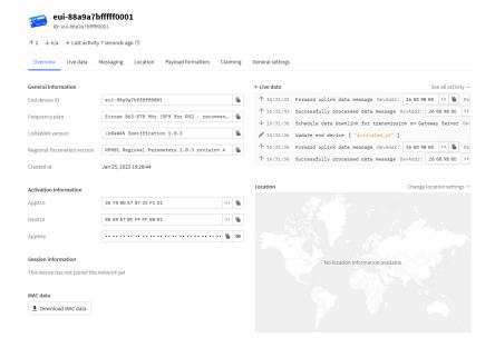
Enter the DevEUI from the nameplate of your device. You also need to enter the AppKey or Network key, which is customer specific and can be found on the connection assignment sheet delivered with each sensor. Finally, press *Register end device*. The device will then start to search for the nearest LoRaWAN access point and connect to the network.
