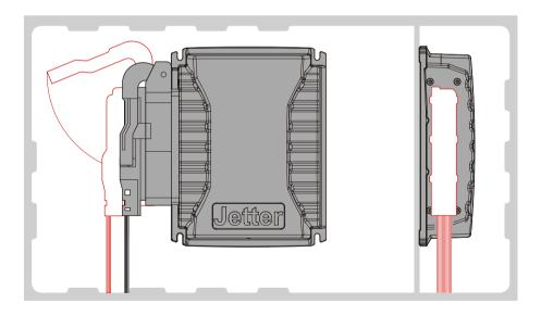
Ensure there is enough space around the connector for servicing requirements. It should be possible to disconnect the connector at any time.
