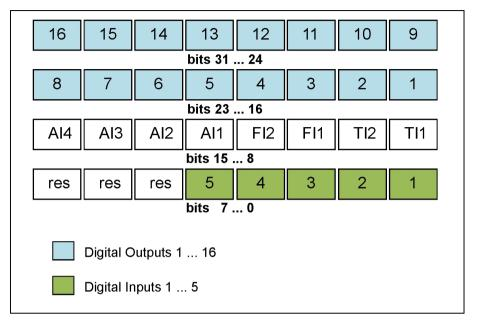
In the diagram, the green bits represent the five digital input channels. The blue bits represent the sixteen digital output read back functions. The other bits are labelled:
