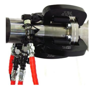
Replacement of damaged nuts – Industrial Clamping
