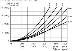
$\Delta p$  = f (Q) Pressure drop - Flow rate characteristic Lowering B  $\rightarrow$  A (through cartridge valve only)
