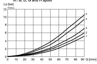
$\Delta p = f(Q)$  Pressure drop - Flow rate characteristic A / B, D, G and H spool
