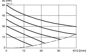
p = f(Q) Pressure - Flow rate characteristic [ $p_N = 160$  bar]  $p_2$  [bar]
