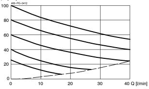
p = f(Q) Pressure - Flow rate characteristic [ $p_N = 250$  bar]  $p_2$  [bar]
