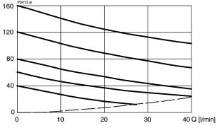
p = f(Q) Pressure - Flow rate characteristic [ $p_N = 100$  bar]  $p_2$  [bar]
