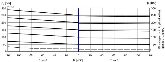
p = f(Q) Pressure - Flow rate characteristic [ $p_N = 350$  bar]
